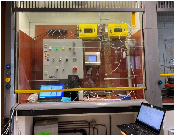
Bench scale bubble column (6L)
